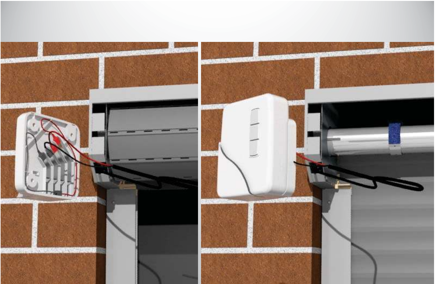
Step 24: Before wiring the DC motor, the roller shutter must be closed to have access to feed the cable into the wall cavity. Connect the motor temporarily by using the battery handset and handset holder to operate and close the roller shutter. [Note: Make sure your battery handset is charged]
