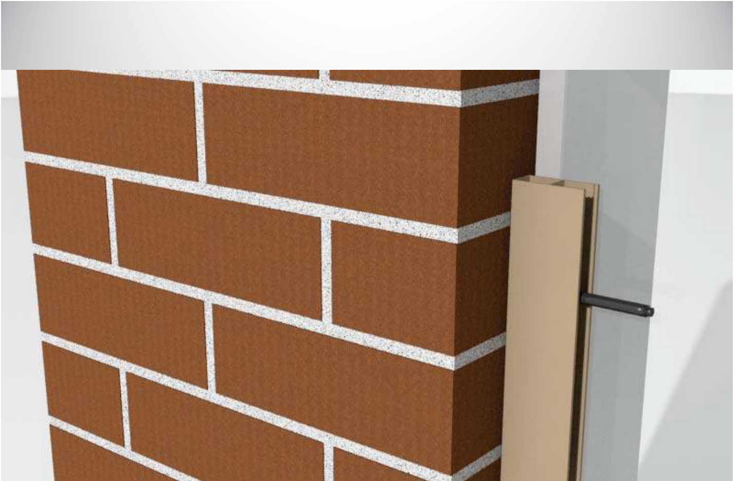
Step 13: Put one of the shutter guides on the wall and mark the holes on the wall.
