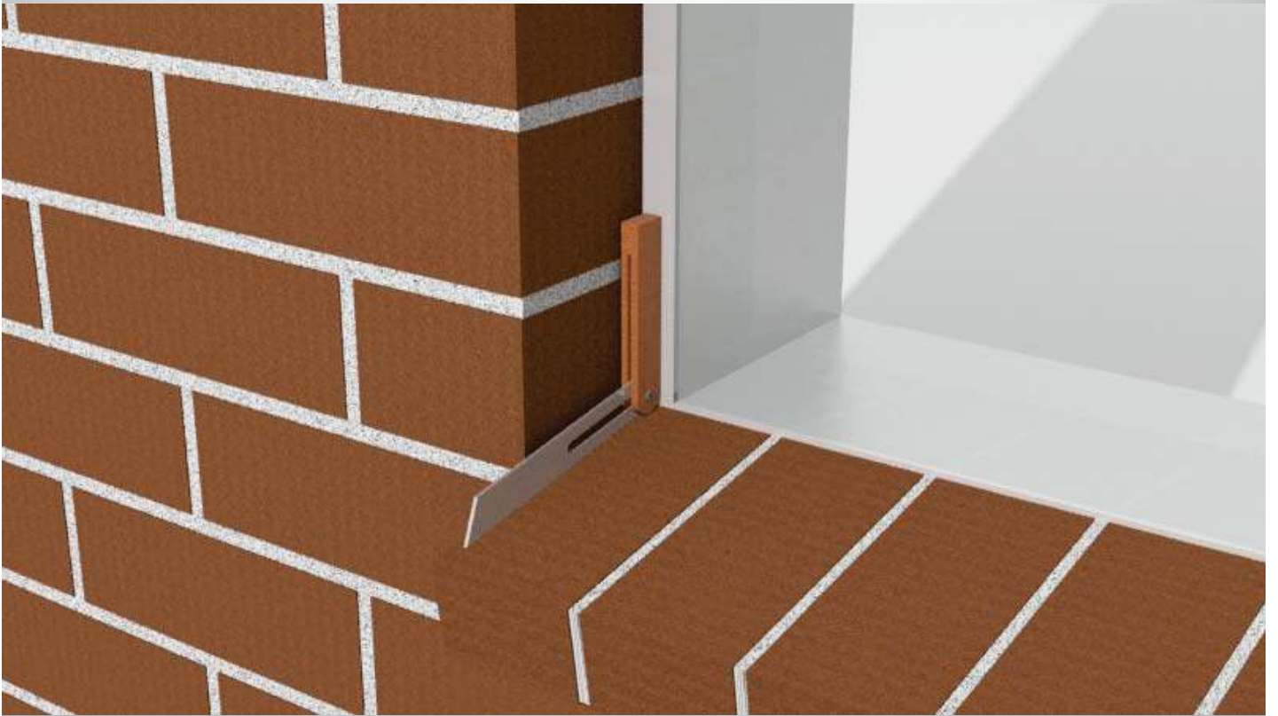
9. Measure the angle of window sill using a bevel
