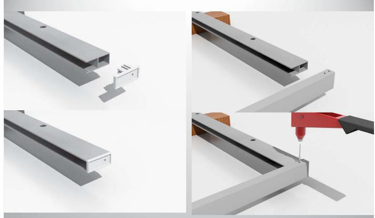
Step 19: Slide the bottom caps in place if sill angle is not required. If sill angle is required, secure the sill angle with supplied rivets in the pre-drilled holes.
