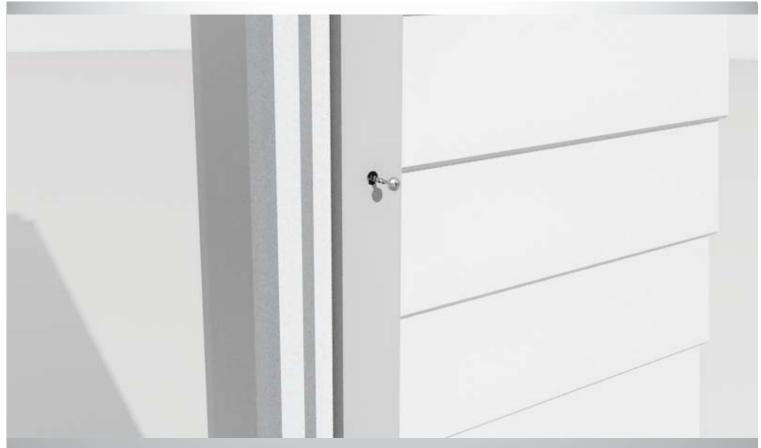
Step 17: Secure the packer on the wall using the provided screws.
