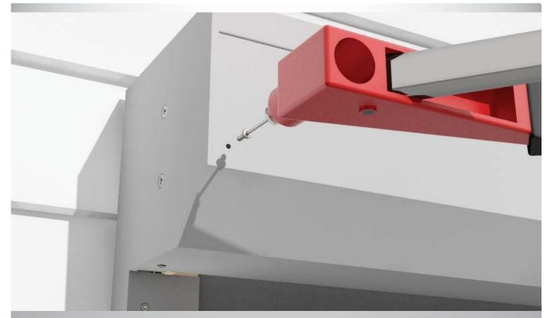
Step 26: Put the front cover in place by sliding it in and securing it using the provided rivets into the pre-drilled holes.
