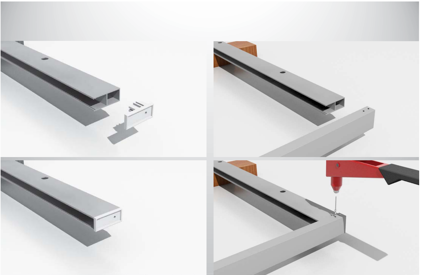
Step 18: Slide the bottom caps in place if sill angle is not required. If sill angle is required, secure it using rivets and pre-drilled holes.
