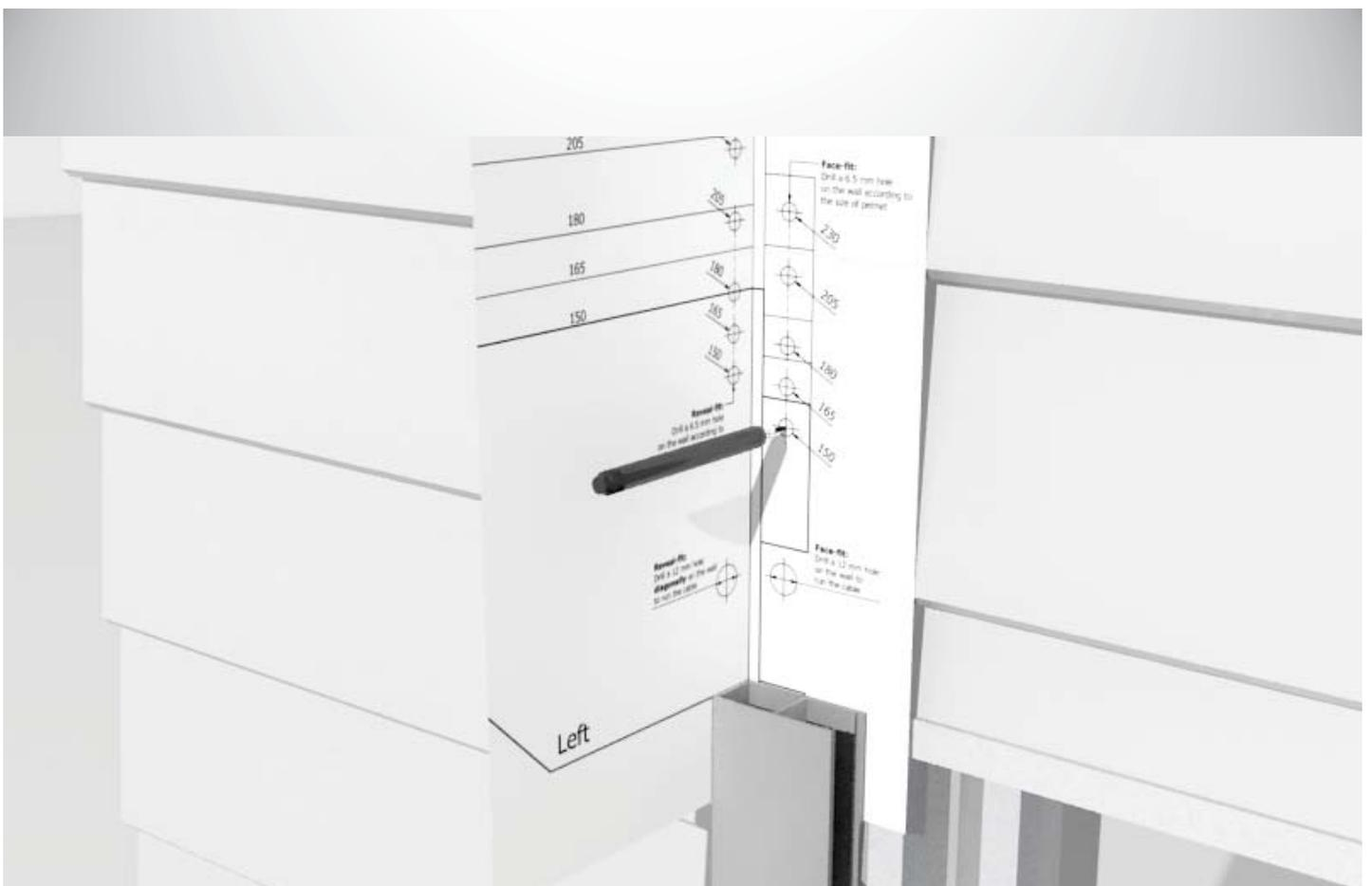
Step 6: Mark the securing point for the pelmet box and the hole for the DC motor cable on the wall. Remember that the hole for the cable is only needed on one side.
