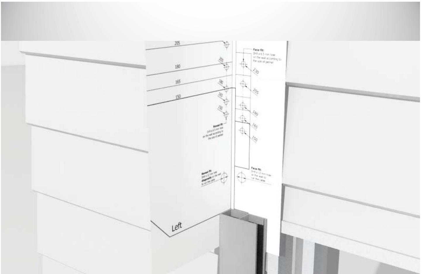
Step 5: Use the proper paper template to estimate the final position of the pelmet box and securing points. Fold the template and place the guide over the shaded area on the paper template.
