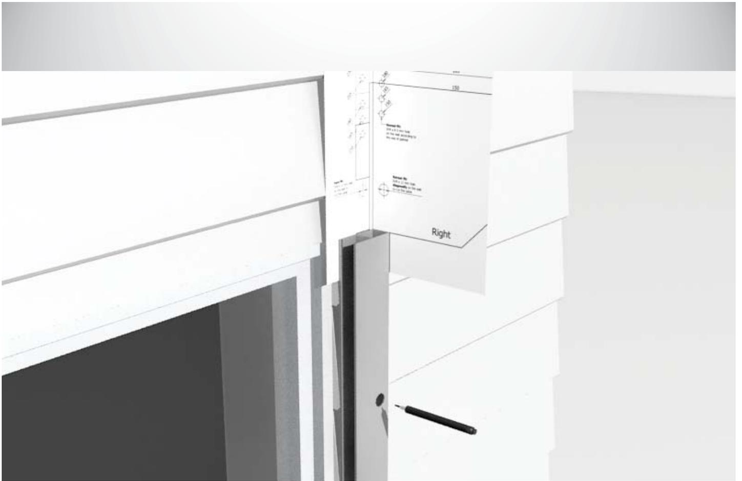
Step 15: Use the template for the other side as well to mark the securing point for pelmet box. Also mark the shutter guide fixing points on the wall.
