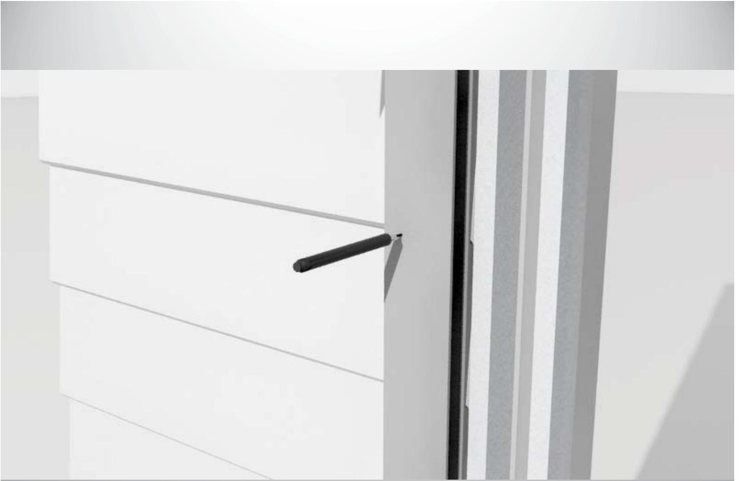
Step 7: Mark at least 3 fixing points on the shutter guide approx. 100 mm from the top and bottom and distribute the holes approx. 400~500 mm apart making sure you place the holes over the bullnose. (the highest point on the timber)
