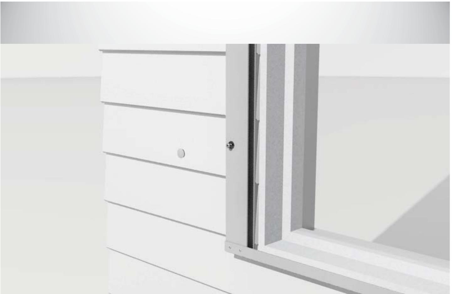
Step 22: Secure the shutter guides using the provided screws.
