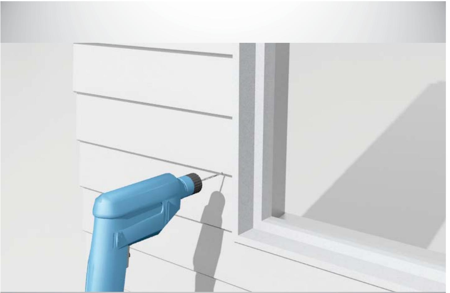
Step 11: Use the 3 mm drill bit to drill pilot holes for securing points including the pelmet box fixing point.
