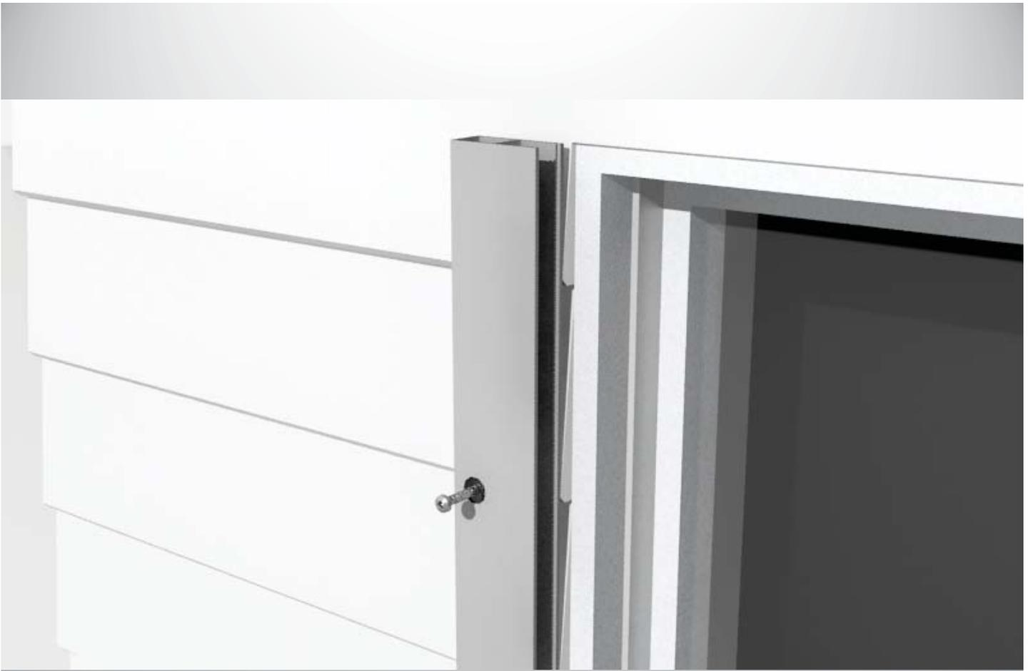
Step 13: Secure the shutter guide temporarily by using just two screws.
