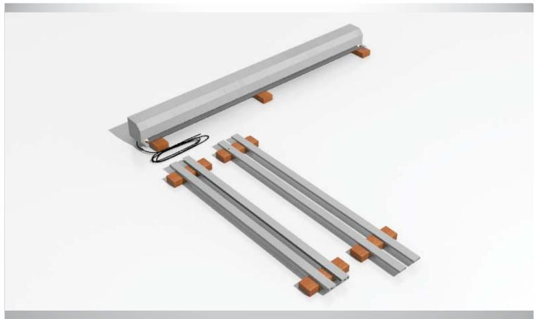
1. Unwrap the pelmet box, guides, and packing profiles and put them on the ground
