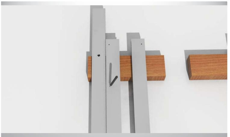
Step 9: Mark at least 3 fixing points on the shutter guides approx. 100 mm from the top and bottom and distribute the holes approx.  $400^{\sim}500$  mm apart, making sure they don't overlap with the packer's holes drilled in the packers.
