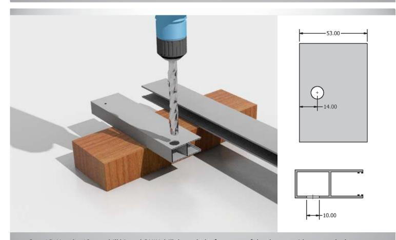
Step 10: Use the 10 mm drill bit and ONLY drill through the front part of the shutter guides on marked positions. Do not drill all the way through.
