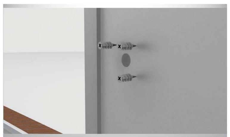
Step 29: Depending on your internal wall type, you may need special plugs for securing the handset holder on the wall.
