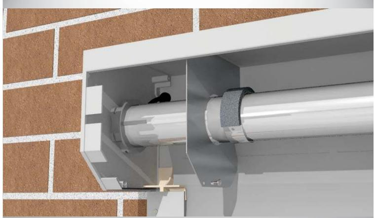
Step 27: With the shutter closed, unscrew the protective plate and slide it over the axle. Feed the wire through the drilled hole into the wall and screw the protective plate back in place.
