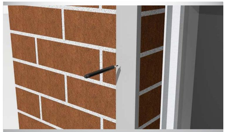
Step 5: Mark at least 3 fixing points on the packer approx. 100 mm from the top and bottom and distribute the holes approx. 400~500 mm apart making sure you do not place the holes where the mortar is.
