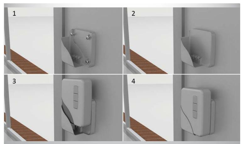
Step 33: Secure the handset holder on the wall and put the cover back in place. Now you can put the battery handset inside the holder and it is ready to use.
