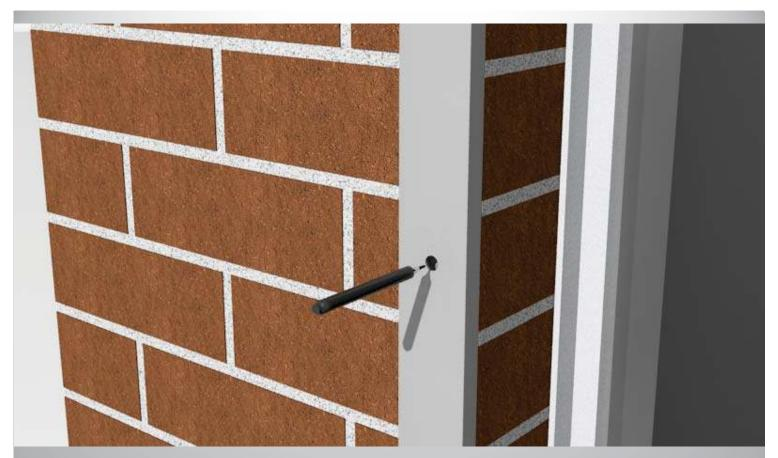
Step 11: Put one of the packers on the wall and mark the holes on the wall.
