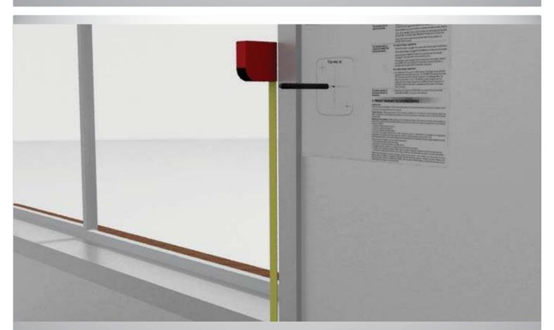
Step 28: Use the provided paper template with the handset holder to mark the centre and fixing points on the wall inside the house.
