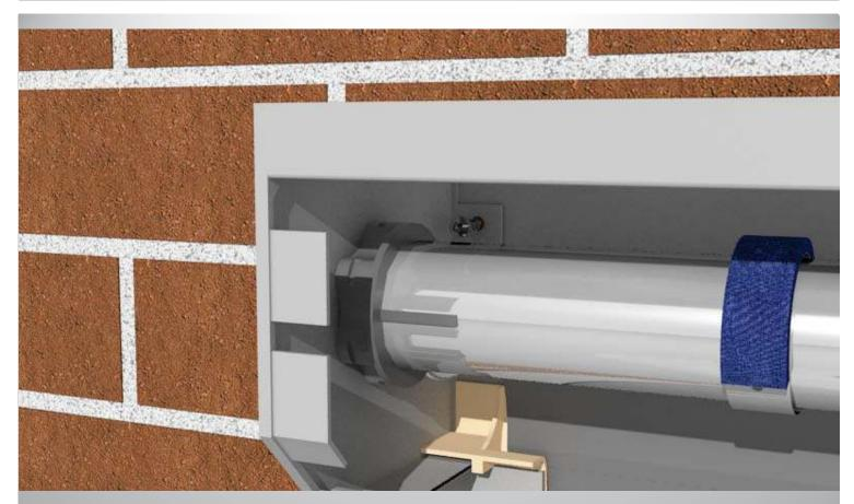
Step 34: With the shutter closed, secure the pelmet box.
