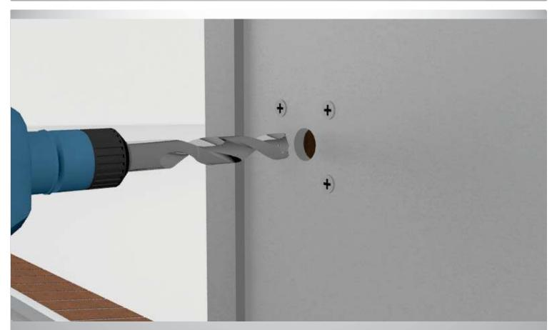
Step 30: Drill a hole in the centre for the cable.
