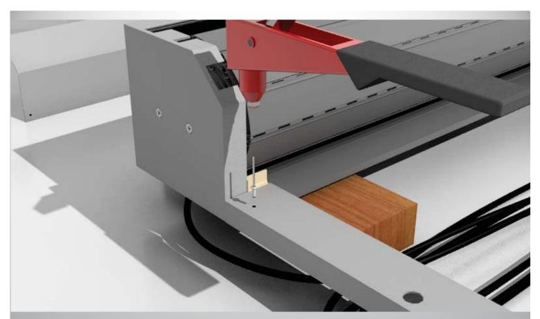
Step 21: Slide the shutter guides onto the end plate legs and secure them with the supplied rivets in the predrilled holes.
