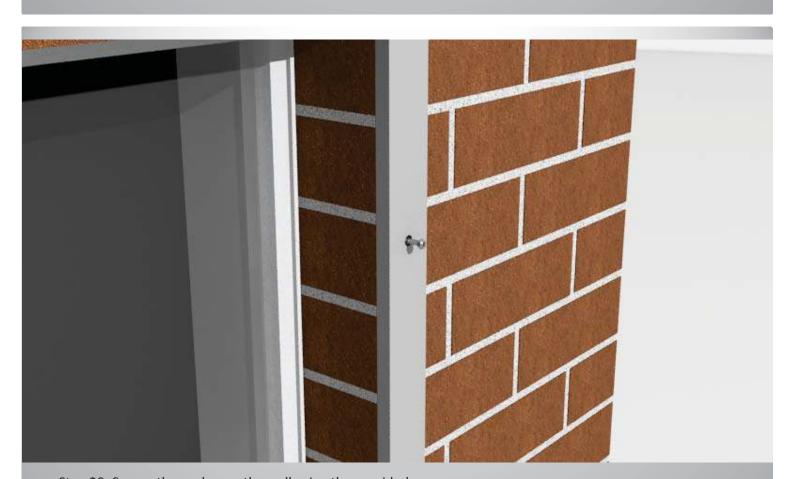
Step 20: Secure the packer on the wall using the provided screws.
