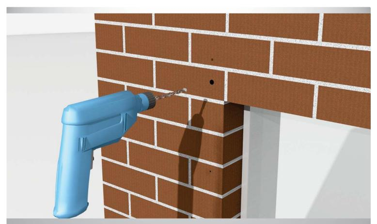
Step 13: Use the 12 mm masonry drill bit to drill a hole for the DC motor cable through the exterior wall to get the cable into the wall cavity. Do not drill through interior wall.
