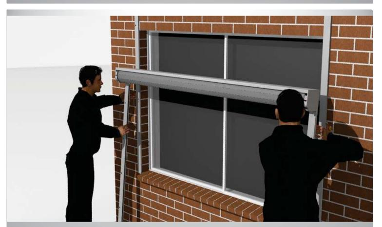
Step 24: For lifting the shutter, two people will need to hold the assembly on both sides and lift at the same time to place it on the wall. Then slide it up in place while pushing against the wall.
