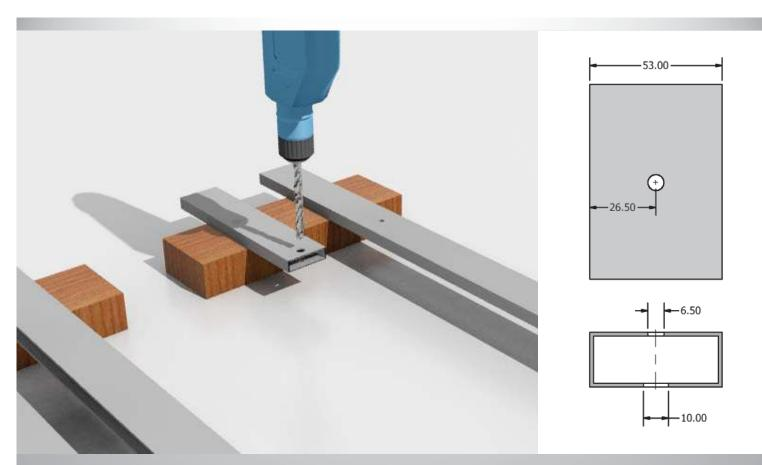
Step 7: Then change the drill bit to 10 mm and ONLY drill through the front part of packer on all holes. Do not drill all the way through.
