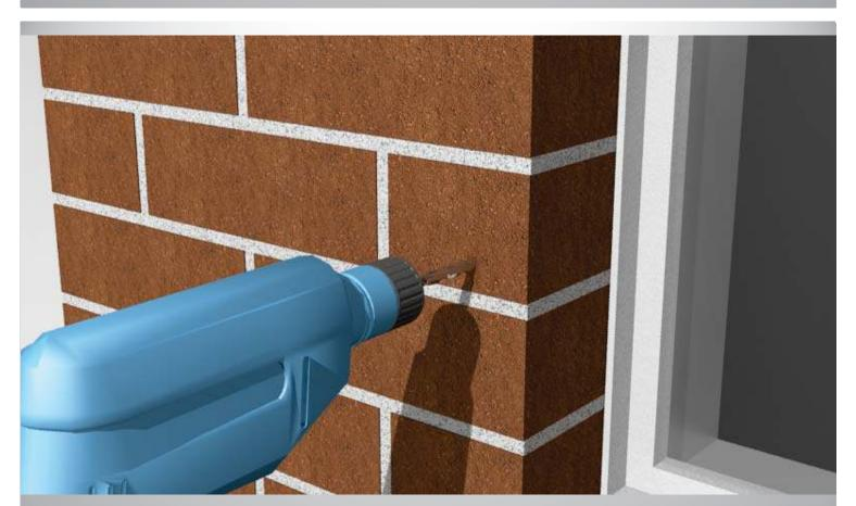
Step 12: Use the 6.5 mm masonry drill bit to drill holes at 35 mm depth on the wall for all fixing points including the pelmet box fixing point.
