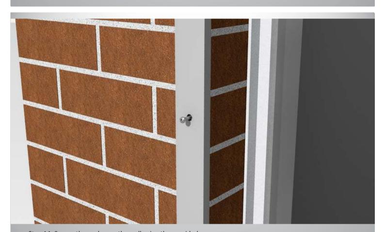
Step 14: Secure the packer on the wall using the provided screws.
