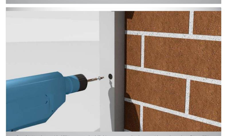
Step 24: Use the provided TEK screws and a drill-driver to secure the shutter guides on the packers. [Note: TEK screws are self-drilling screws and don't need additional holes pre-drilled before use.]
