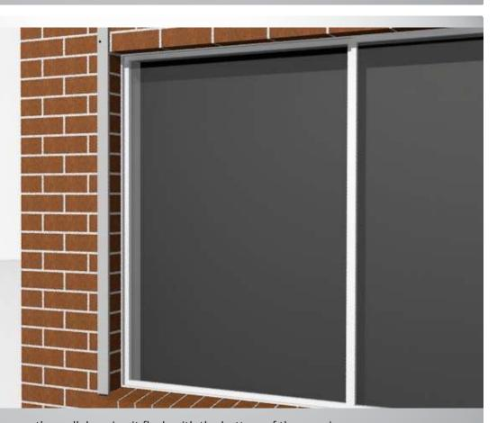
Step 4: Place one of the packers on the wall, keeping it flush with the bottom of the opening.
