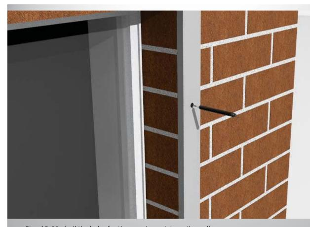
Step 16: Mark all the holes for the securing points on the wall.
