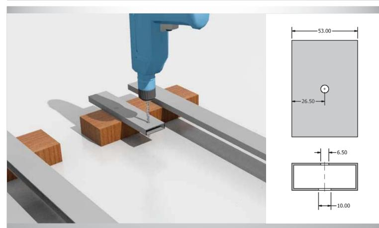
Step 6: Put the packer back on the ground and use the 6.5 mm drill bit to drill the holes all the way through on the points you have marked. Do the same on the other the packer.
