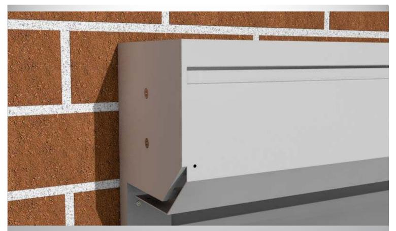
Step 27: Put the front cover in place by sliding it in and securing it using the provided rivets into the pre-drilled holes.
