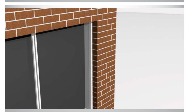
Step 18: Put the wall plugs in place for fixing points.
