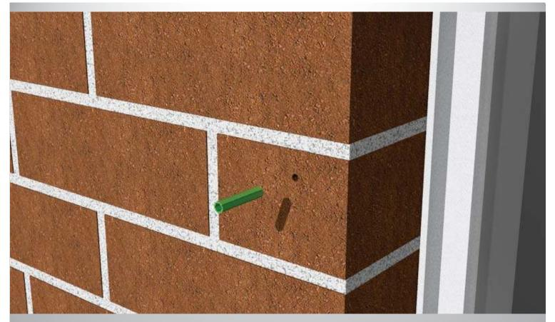
Step 13: Put the wall plugs in place for fixing points.
