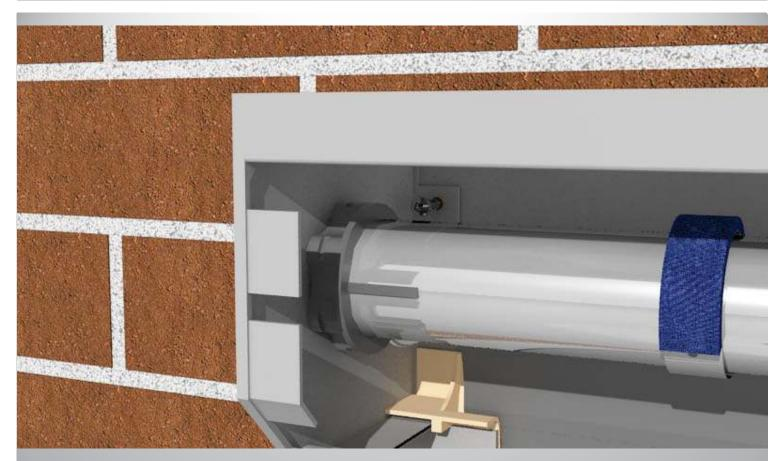
Step 26: With the shutter closed, secure the pelmet box.
