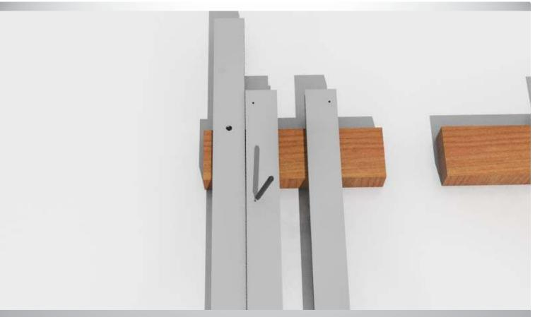
Step 9: Mark at least 3 fixing points on the shutter guides approx. 100 mm from the top and bottom and distribute the holes approx. 400~500 mm apart, making sure they don't overlap with the packer's holes drilled in the packers.
