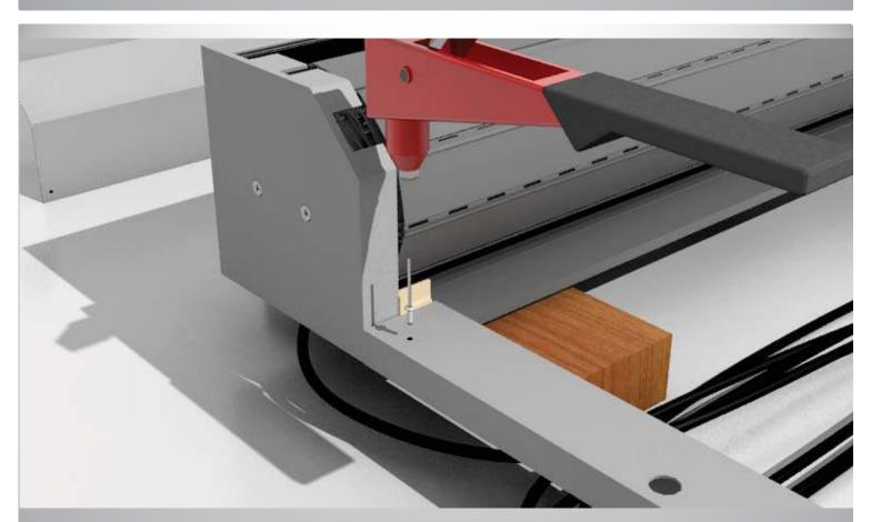
Step 20: Slide the shutter guides onto the end plate legs and secure them with the supplied rivets in the predrilled holes.
